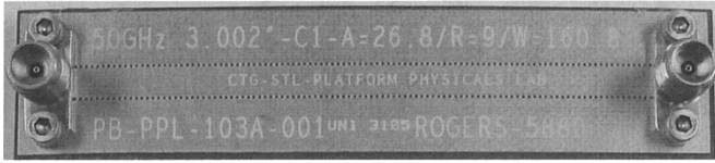
Fig. 4. 7.6-cm-long SIW interconnect scaled to a center frequency of 50 GHz. This test structure is comprised of Rogers RT/Duriod 5880 dielectric material ( \epsilon_r = 2.2 and \tan \delta = 0.0009 ) and has r = 0.24 mm, a = 0.68 mm, w = 4.1 mm, and h = 0.76 mm. Further, it is 35% smaller in the transverse direction than the EBG waveguide of Fig. 2.
