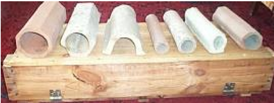
Figure 1. Drain tile shapes.
