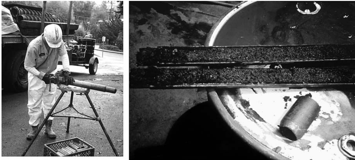
Figure 4. A split-spoon sampler barrel must be recovered from the hole, detached from the drill rod, and mechanically broken down, as shown at left. The two halves of a typical Standard Penetration Test (SPT) sampler with entrained soil are shown at right.
