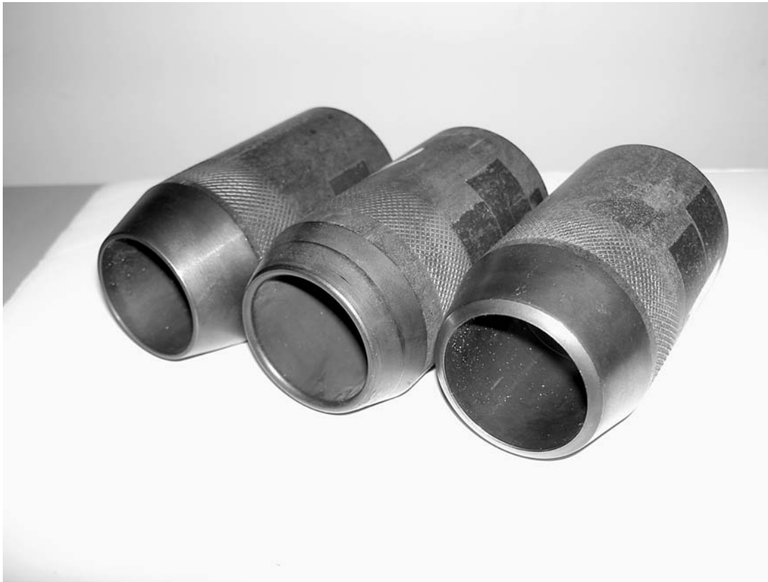
Figure 3. Drive samplers usually employ three types of cutting heads, or shoes, shown here. The sharp tapered heads are intended for soil sampling, while the more blunt tips are designed for greater longevity when sampling granular soils.
