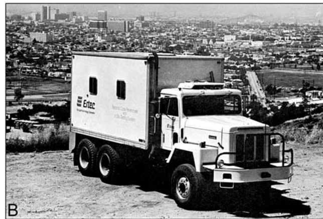
Figure 12. (A, left). Cone tip exposed beneath truck, just before being advanced into the ground at a rate between 1 and 2 cm/s. The cone has an area of either 10 or 15 cm 2 and is typically advanced in 1-m increments because the rods are of that length. (B, right) A Hogentogler Cone Penetrometer Test (CPT) rig operated by Ertec in Long Beach, CA. Truck-mounted rigs weigh about 18 tons and are capable of exerting considerable normal force on the advancing rods.
