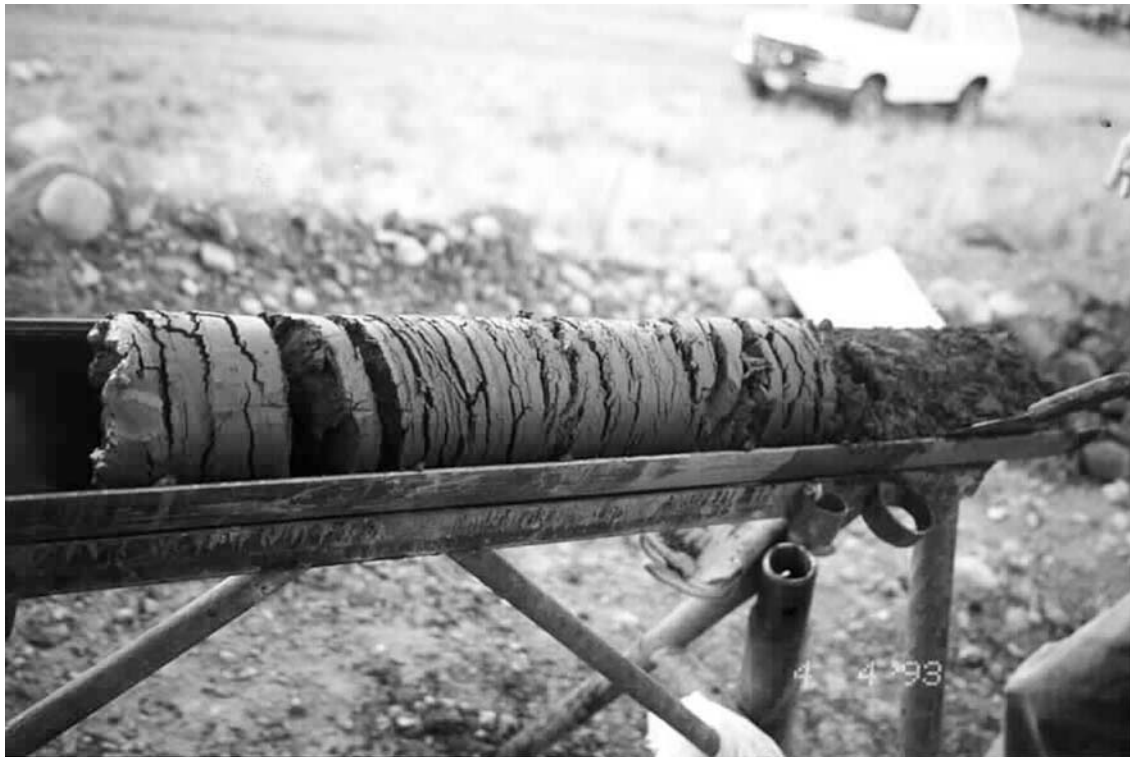
Figure 9. Five-inch (12.7-cm)-diameter drive sample of soil in an embankment dam recovered using a hollow stem flight auger drill rig. Note disturbance caused by multiple tensile separations. Image courtesy of Jeffrey A. Farrar, U.S. Bureau of Reclamation.
