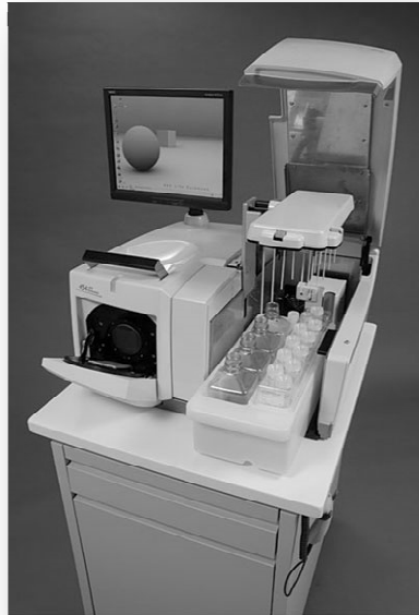
Figure 8. The 454 Genome Sequencer instrument based on the 454 sequencing technology, including the pyrosequencing principle. (Source: Blow, 2007. Rights of 454 Sequencing © 2010 Roche Diagnostics)
