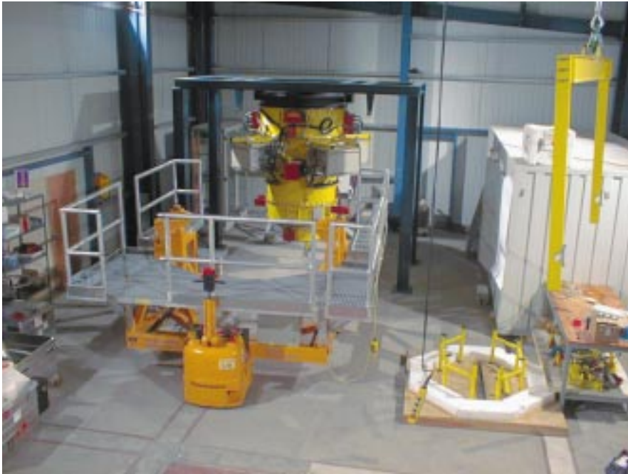
Figure 3: Re-assembly in the Auxiliary Telescope Hall on Paranal with FORS1 on the integration stand in the background, the control cabin at right and the Cassegrain carriage (foreground left) which is used for all major transport and handling operations.
