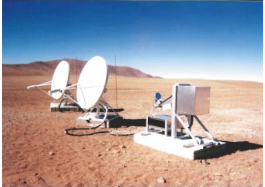
Figure 4: One of the 183-GHz water vapour monitors to the right of the antennas of the 11.2-GHz interferometers.
