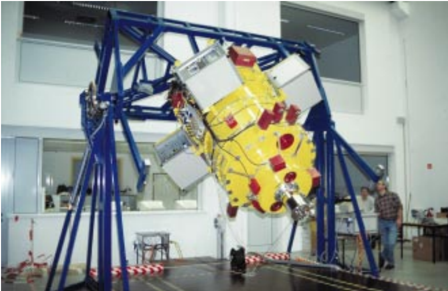
Figure 2: FORS1 on the telescope simulator during flexure tests in the integration hall of DLR at Oberpfaffenhofen near Munich.
