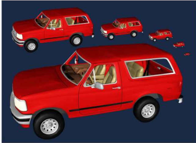
Plate 1: 6 views of the Ford Bronco model, all at 2 pixels of error (0.17 mm)
