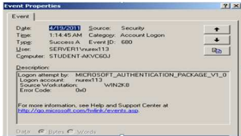
Fig (5.2): Event ID 680 recorded when the attacker successfully logon to the victim system
