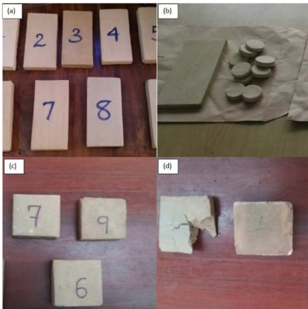
Figure 2. Disc- and tile-shaped bodies fabricated using vermiculite and RHA for physical and mechanical properties tests (a) green bodies (b) fired bodies (c) fired and labelled bodies (d) fired bodies with visual defects such as cracks, lamination and surface deformation.
