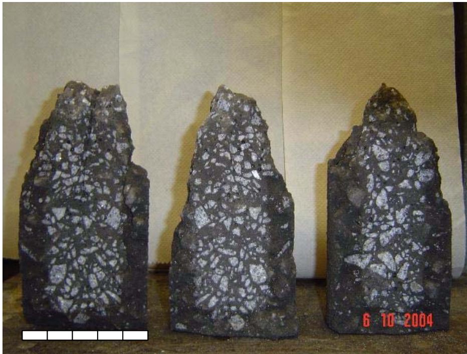
Figure 10 Penetration of sulfuric acid after 1 year of exposure
