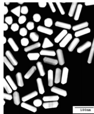
Figure 6. TEM image (Philips CM-10, 80 kV) of anisotropic Au nanoparticles prepared in the absence of AgNO 3 , followed by quenching with Na 2 S ( t = 25 min). Nanorod suspensions were subjected to one C/R cycle prior to sample preparation.
