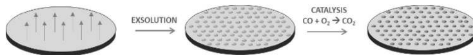
Fig. 1 Model catalyst samples. Schematics of exsolution of metallic nanoparticles at the top surface of dense pellet perovskite oxide samples. Before and after the catalytic tests the pellet is loaded in the
