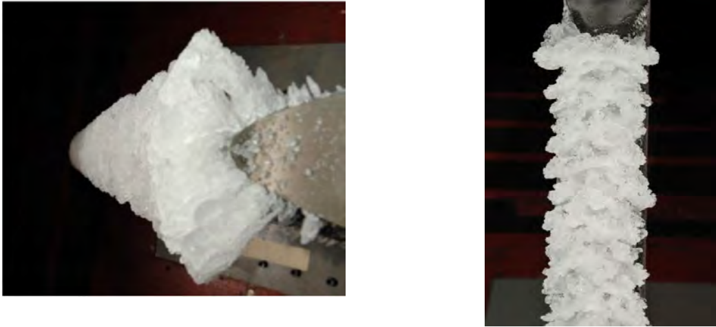
Fig. 21 Spanwise and frontal views of experimental ice accretion, case 372 (glaze) [7].
