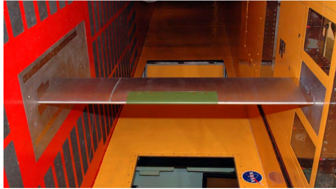
Fig. 10 36-inch NACA23012 Airfoil in icing tunnel (rotated) [4].
