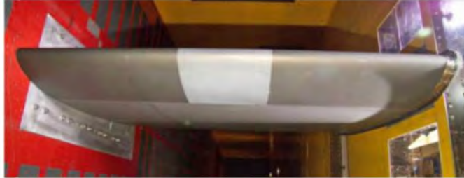
Fig. 15 72-inch NACA23012 Airfoil in icing tunnel (rotated) [5].
