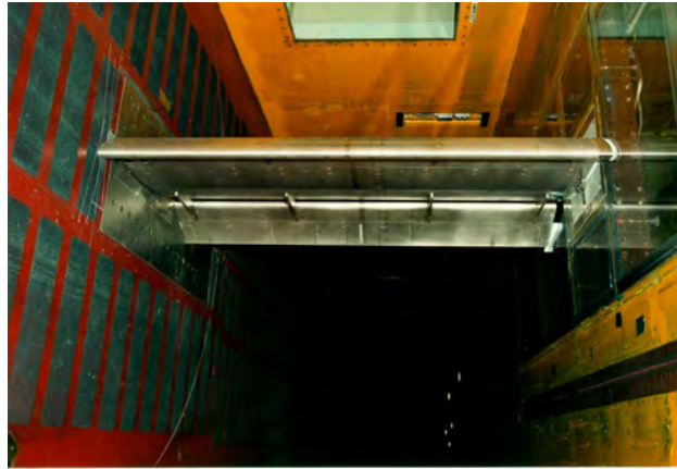
Fig. 3 Case 121/122 three-element airfoil in icing tunnel (rotated, downstream) [2].
