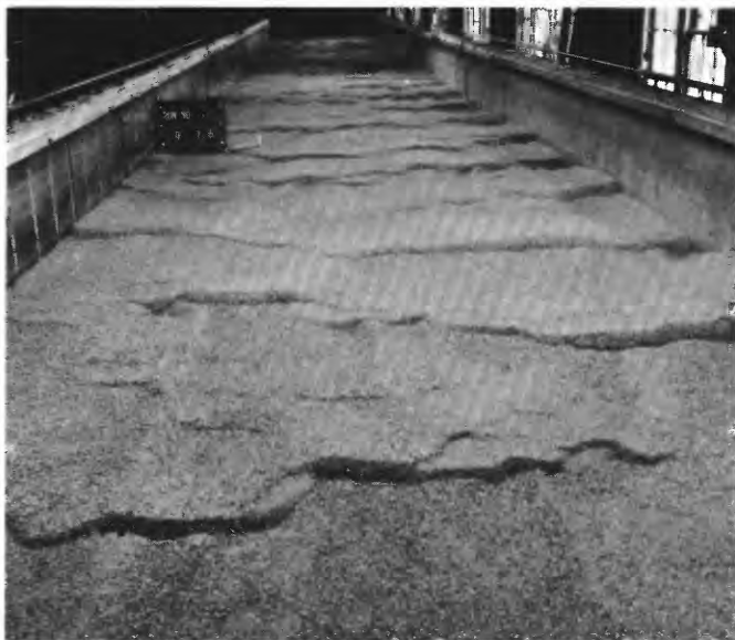
FIGURE 62.—Upstream view of the dune-bed condition at the end of run 35.
