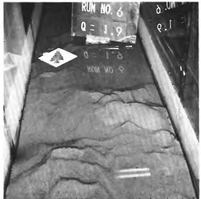
FIGURE 72.—Downstream view of dune-bed configuration formed during run 6.
