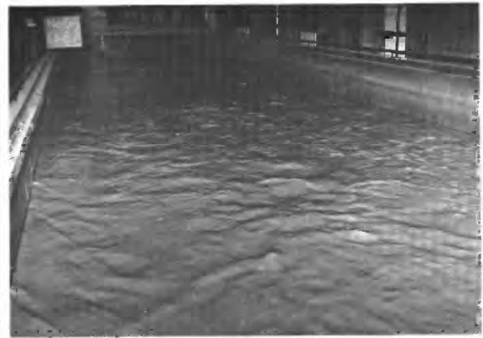
FIGURE 91.—Upstream views of the water surface during runs 51 (A) and 96 (B) contrasting the increase in turbulence with increased flow stress and resistance.
