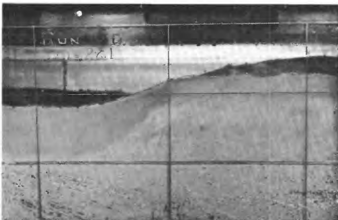
FIGURE 26.—Flow and bed characteristics of antidune conditions during run 19, photographed through window in side of the flume. A, The trough of a water wave. B, The upstream side, or deceleration area, of a wave. C, A breaking wave, showing heavy concentration of suspended sand.
