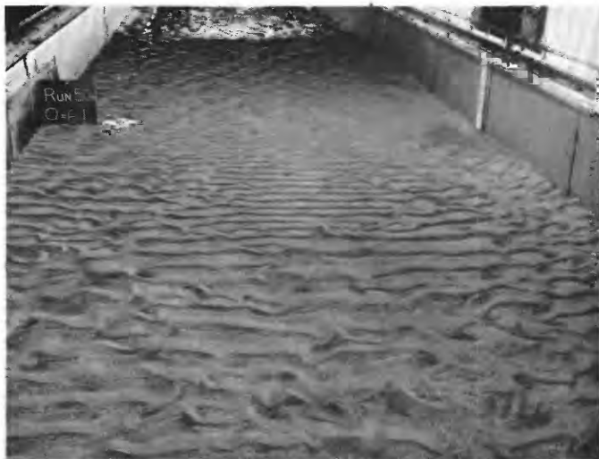
FIGURE 31.—Upstream view of ripples on the bed of the flume at the end of run 50D.
