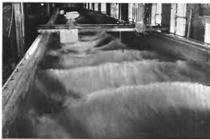
FIGURE 57.—Flow conditions during run 32. A , View downstream showing train of antidunes near station 80. B , View upstream from station 125 showing large antidunes occupying full width of flume, and narrower antidunes from station 95 to the head of the flume.
