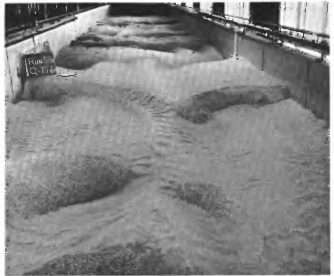
FIGURE 34.—Upstream view of the bed configuration at the end of run 53.
