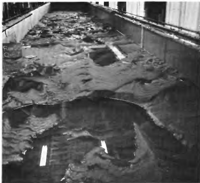
FIGURE 39.—Upstream view of the bed configuration at the end of run 58.
