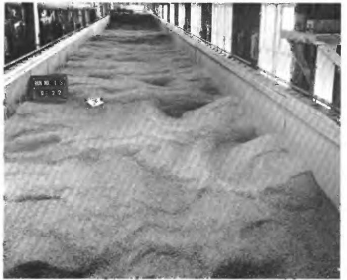
FIGURE 68.—Upstream views of flow and bed conditions for run 13. A, Water-surface condition. B, Bed configuration at end of run.
