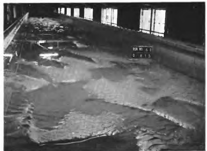
FIGURE 21.—Upstream view of ripples on low dunes characteristic of run 6. The pools of water remained after incomplete drainage at the end of the run.
