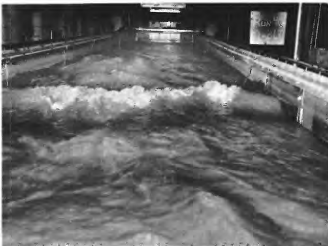
FIGURE 40.—Downstream view of water-surface conditions during run 48. Note the breaking antidune near the center of the flume.
