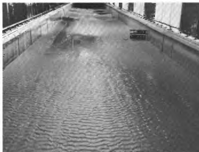
FIGURE 16.—Typical bed conditions at end of run 13. The small surface waves were caused by slow flow at the time of shutdown.
