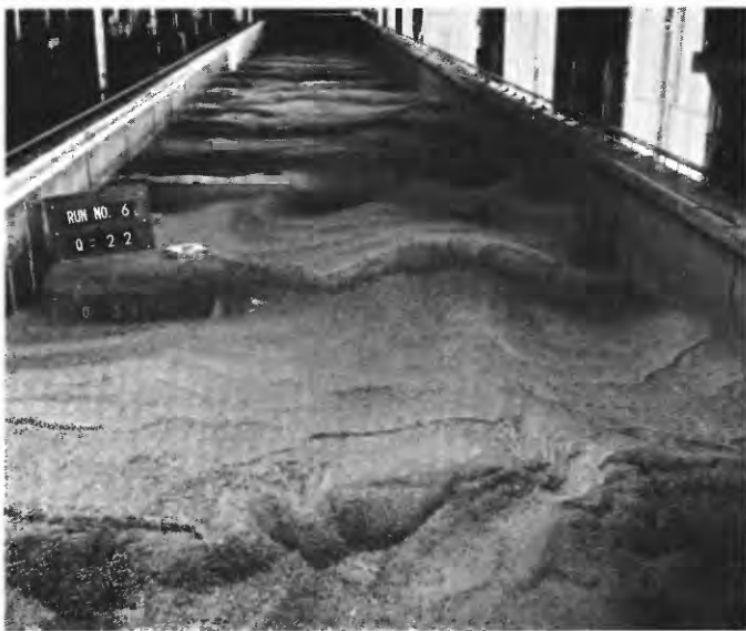
FIGURE 65.—Upstream view of the dune-bed configuration formed during run 6.
