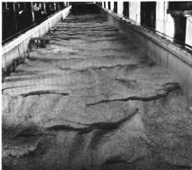
FIGURE 64.—Upstream view of the dune configuration at the end of run 10.
