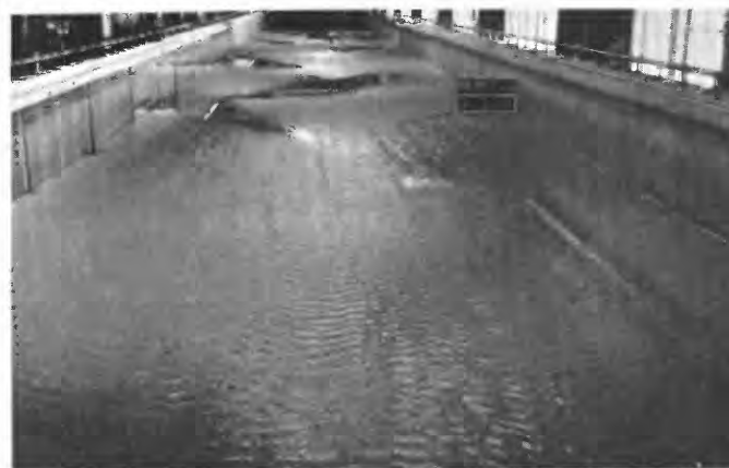
FIGURE 17.—Upstream view of bed conditions at the end of run 14. The small surface ripples formed during shutdown.
