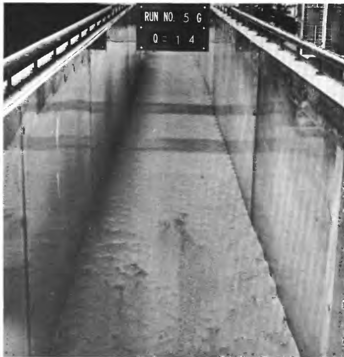
FIGURE 82.—Upstream view of ripples formed during run 5.
