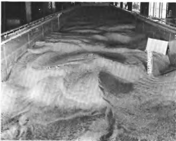
FIGURE 52.—Upstream view of the dune-bed configuration at the end of run 21.
