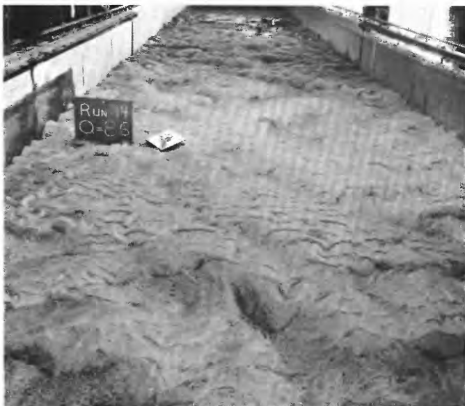
FIGURE 44.—Upstream view of the dune-bed configuration at the end of run 14.
