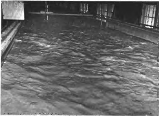
FIGURE 93.—Upstream view of water surface during run 95. The flow, at a velocity of 2.39 fps, is over a dune-bed form.
