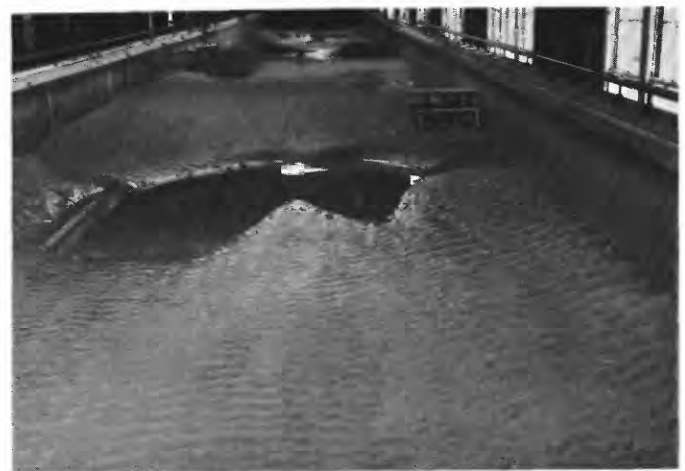
FIGURE 20.—Bed configuration at the end of run 12, viewed upstream. Note large rather streamlined dunes.
