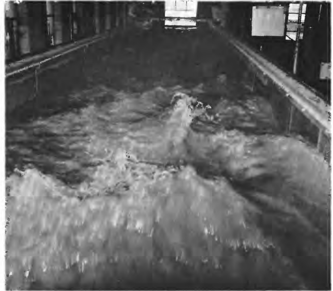
FIGURE 41.—Downstream view of flow conditions (chute-and-pool flow) during run 40.
