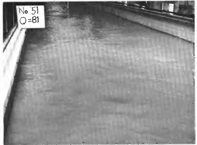
FIGURE 89.—Ripples and lenses of fine material (light colored) in the bed during run 88. The relatively round shape of the ripples can be contrasted with the normal-shaped ripples shown in figure 33.
