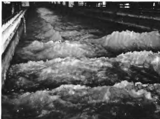
FIGURE 99.—Upstream views of standing waves (A) and breaking antidunes (B) during run 84.
