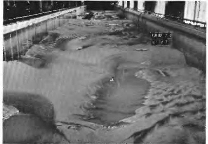
FIGURE 23.—Upstream view of bed configuration at the end of run 7.
