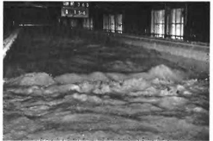
FIGURE 29.—Upstream view of chute-and-pool flow conditions during run 36. Note the air bubbles on the water surface downstream from the hydraulic jump in the foreground of the picture.
