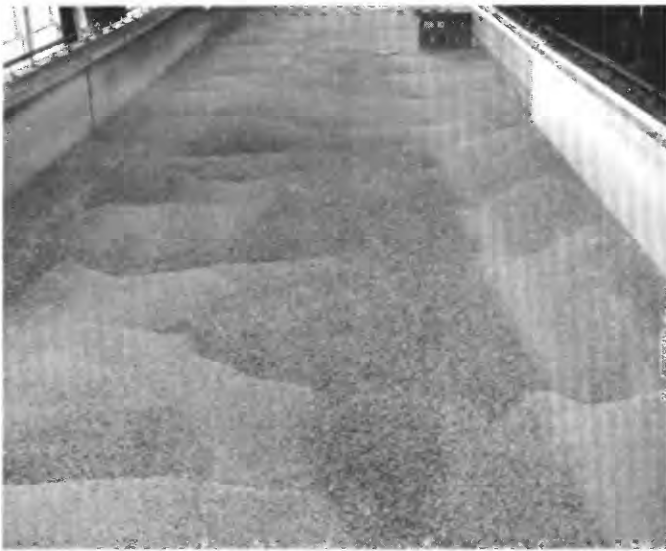
FIGURE 59.—Flume bed at end of run 14. A, View upstream. B, View downstream. Note in view B that the finer material is in the areas of maximum dune height.
