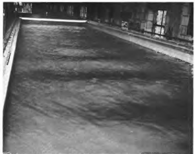
FIGURE 24.—Upstream view during run 16, taken from station 140. Standing waves can be seen in the part of the flume downstream from station 110, and plane conditions, upstream from station 110.
