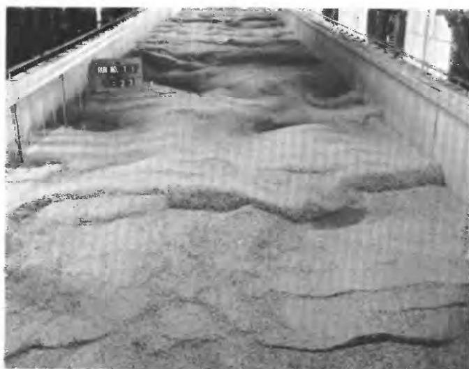
FIGURE 66.—Upstream views of the flow conditions for run 11. A, The water surface. B, The bed configuration at the end of the run.
