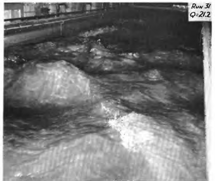
FIGURE 49.—Downstream view of antidune flow conditions during run 31.
