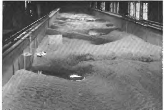
FIGURE 45.—Upstream view of the dune-bed configuration at the end of run 20.
