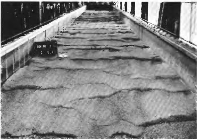
FIGURE 63.—Upstream view of low dunes on the flume bed at the end of run 33.
