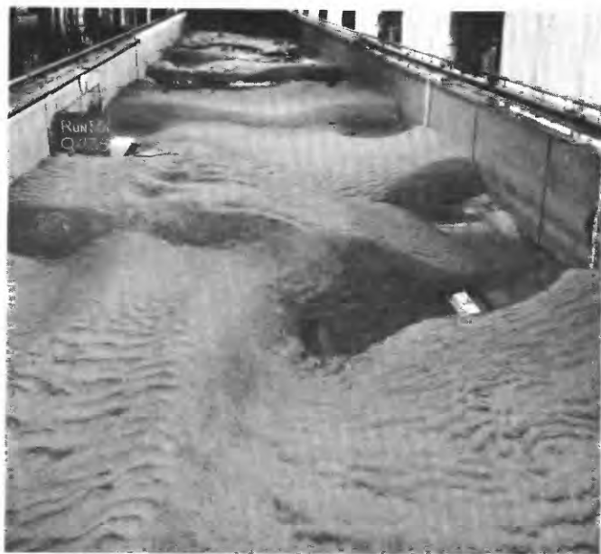
FIGURE 36.—Upstream view of bed configuration at the end of run 55. Note the large dual fins in the left foreground.
