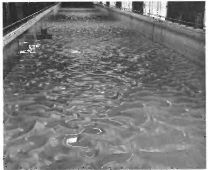
FIGURE 7.—Longitudinal upstream view of the flume bed, showing ripple formation at end of run 2 after slowly draining the water from the flume.
