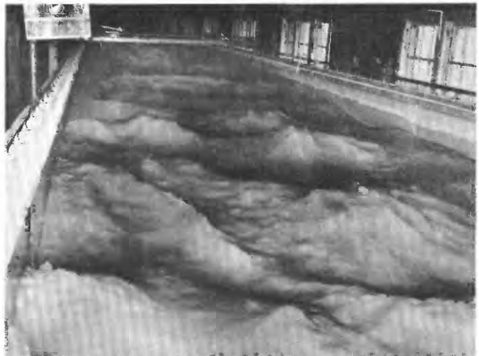
FIGURE 27.—Upstream view of antidune wave pattern during run 21.
