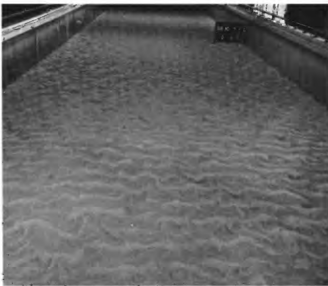
FIGURE 9.—Upstream view of ripples formed during run 25. Ripples are smaller and more completely developed than those formed in run 2 (figs. 7, 8).
