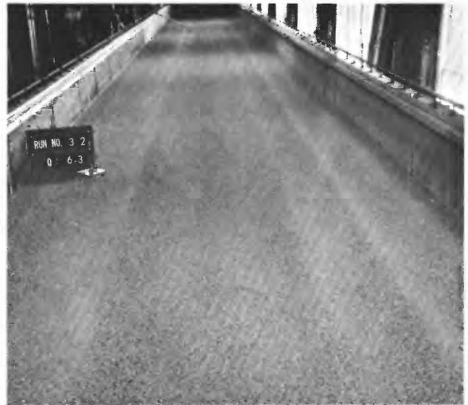
FIGURE 60.—Upstream view of the plane bed at the end of run 32.
