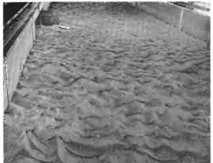
FIGURE 43.—Upstream view of the rippled bed form at the end of run 4.
