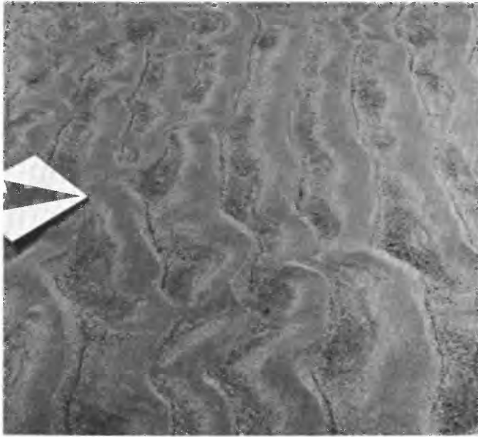
FIGURE 42.—Transverse view of rippled bed pattern at the end of run 9. Note the armor plate of coarse material in the ripple troughs and the rather regular transverse pattern of the ripples.
