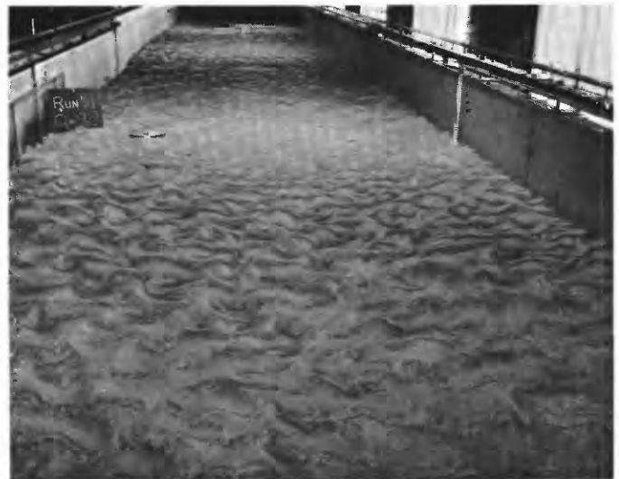
FIGURE 32.—Upstream view of ripples on the bed at end of run 51. Note that the ripples are better developed than those shown in figure 31.
