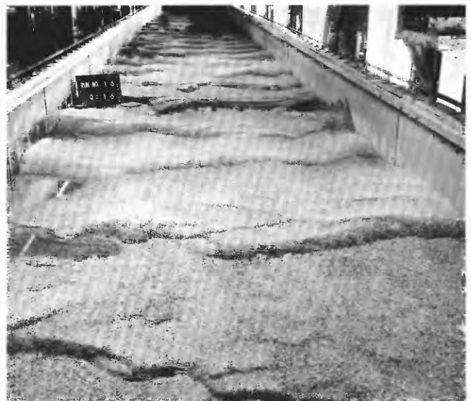
FIGURE 61.—Upstream view of dunes formed during run 16.
