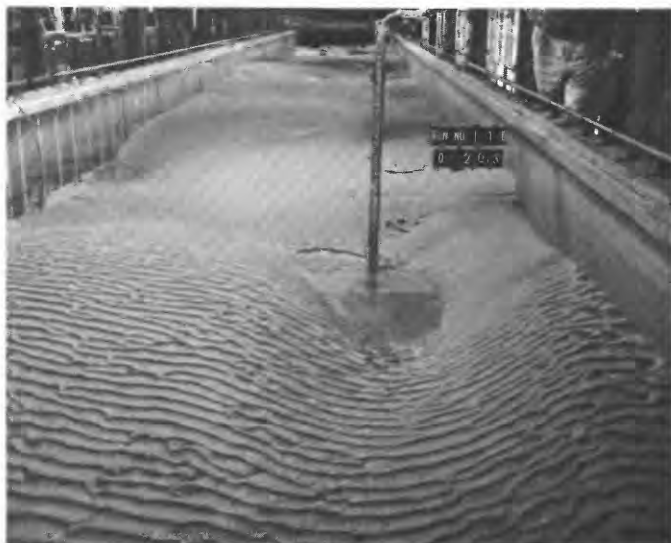
FIGURE 15.—Upstream view of bed configuration at end of run 11. The small surface ripples formed during shutdown of the run. Note the scour hole to the floor of the flume in the foreground.
