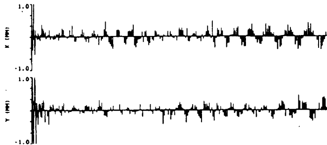
Fig. 7 Empirically determined linac trajectory along the 3 km linac which cancels the errors from the accumulation of dispersion and transverse wakefields errors at 3 \times 10^{10} electrons. This oscillation lowered the horizontal emittance from 4.5 to 3.0 ( \times 10^{-5} r-m). This trajectory is not unique as other trajectories with similar oscillations can produce the same effect.
