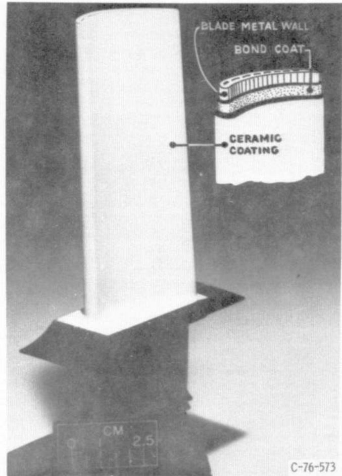
Figure 24. - Ceramic coated turbine blade.
