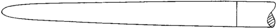
Figure 18. Quartic Body of Revolution geometry. 8 The model is defined as the nose to shoulder, which is 2 inch long.
