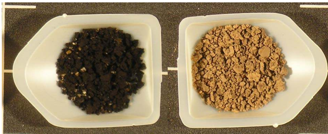
Figure 21. Silver-functionalized Silica Aerogel before (left) and after (right) Maximum Sorption Test.
