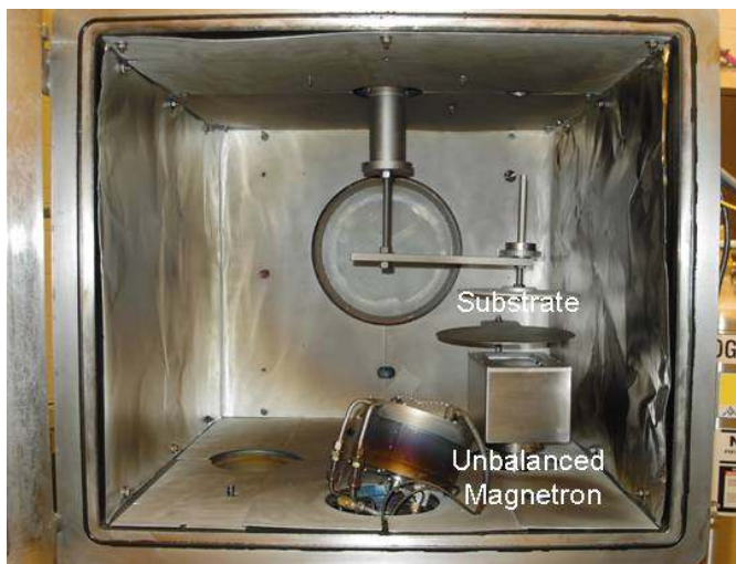
Figure 27. Unbalanced magnetron setup used for several Kr immobilization experiments
