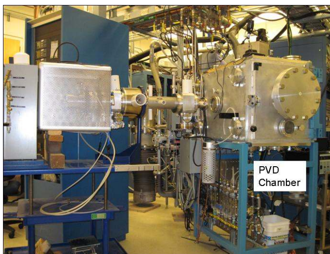
Figure 30. Peabody Scientific ion implanter system (at left) attached to PVD deposition chamber (at right). The implanter is capable of beam energies from 2 to 40 keV with a Duoplasmatron ion source and low-pressure arc discharge system.
