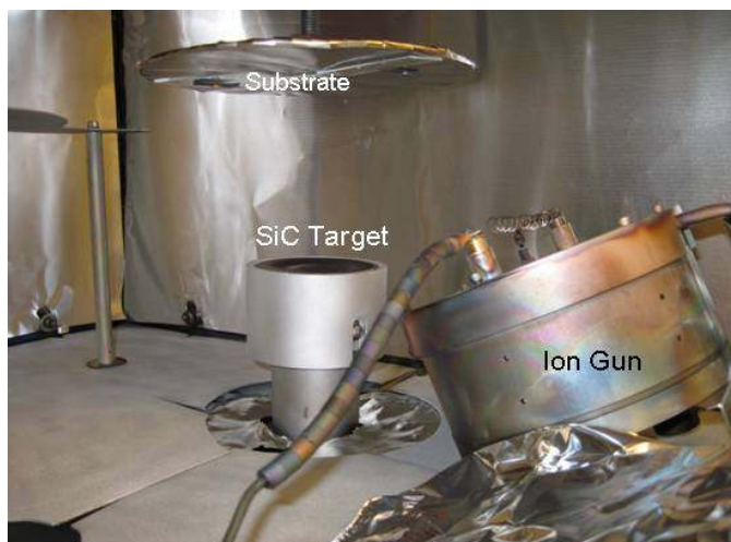
Figure 26. Initial ion gun deposition setup for SiC immobilization experiments with Kr.
