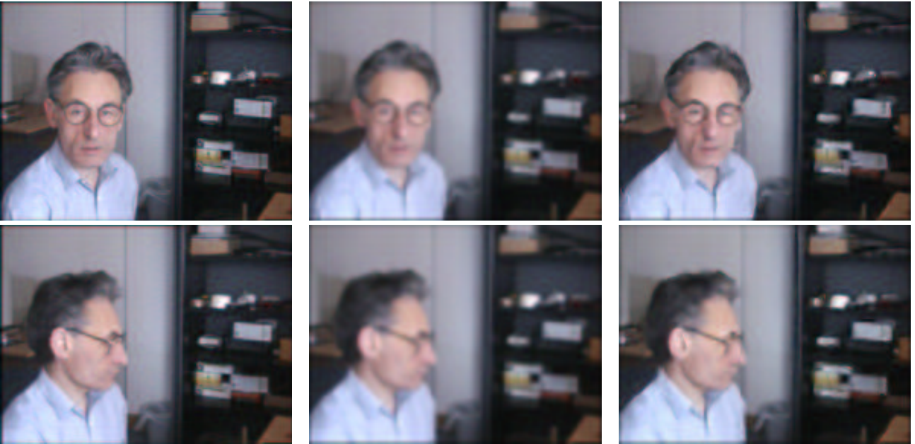
Figure 1: Examples of two frames from a test video sequence showing the original frames (left), the low plus medium frequency components which form the input to the super-resolution algorithm (middle), the output of the super-resolution algorithm (right).
