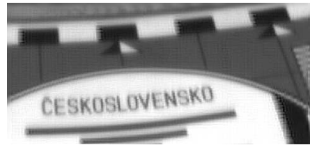
(d) Reconstruction at 5\times zoom with polygon interpolation. This operator has a variable size footprint, and is therefore capable of handling any size zoom factor.
