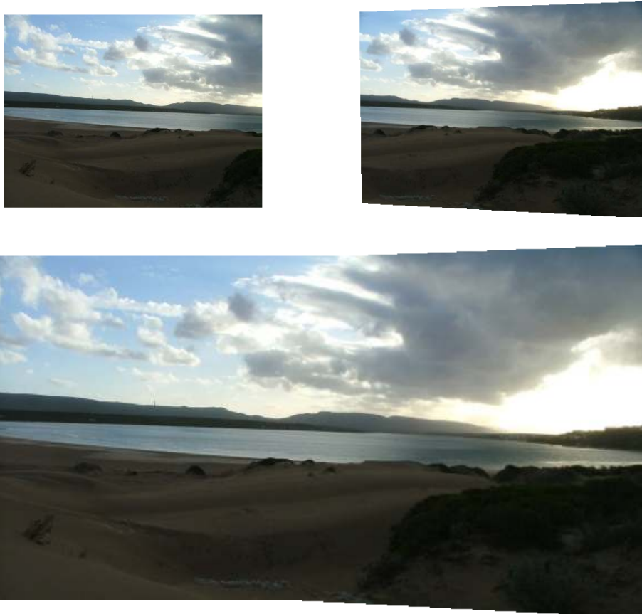
Figure 5.2: Panoramic stitch of two photos. Features are extracted, using the discrete pulse transform, whereafter RANSAC is used to find a homography that fits inliers. The images are warped accordingly (top, left and right) and blended according to a Laplacian pyramid scheme (bottom) (we use the Enblend package; the algorithm is detailed at http://enblend.sourceforge.net/details.htm ). Photos taken at location 34^{\circ}23'52.00''S , 20^{\circ}50'52.09''E .
