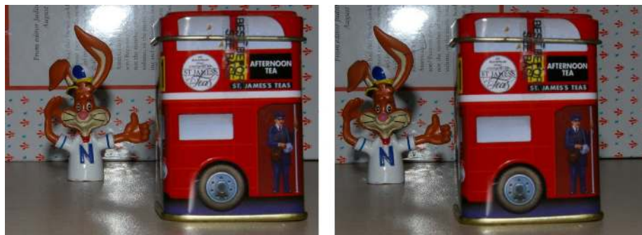
(b) The camera is rotated around a point nearby the pivot point. Parallax is noticeably reduced.
