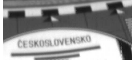
(b) Reconstruction at 5\times zoom with bi-linear interpolation. A high-resolution reconstruction is made, but the result is oscillatory due to the bilinear operator's small footprint.
