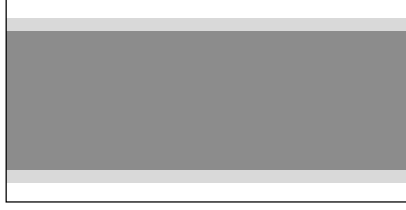
Figure 6: Structure of the numerical domain: In the center strip the random medium is at full strength (75% of the thickness), then there is a smooth transition layer (5–10%) where the strength decreases. In the outer layer the medium is homogeneous, allowing for effective implementation of Discrete Transparent Boundary Conditions.
