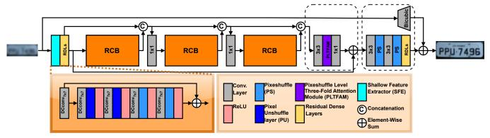
Fig. 1. The proposed architecture, which incorporates an autoencoder consisting of PS and PU layers for feature compression and expansion, respectively. The aim of this design is to eliminate less significant features. In addition, the TFAM modules in the original architecture were replaced with PLTFAM modules throughout the network. The legend inside the figure provides explanations for the acronyms used.
