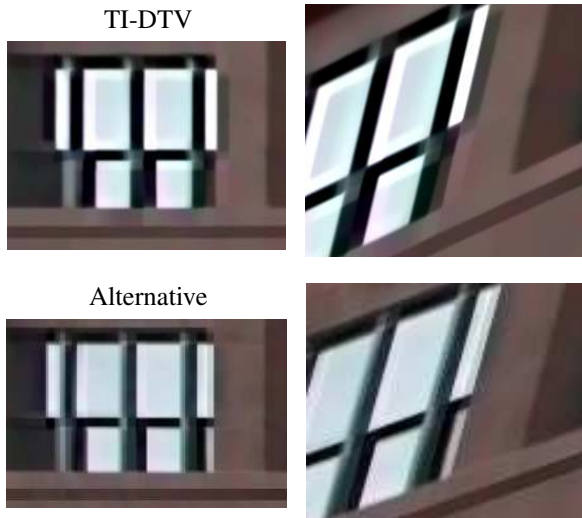
Figure 7. Comparison between solving Problems (2.5) and (2.6) to super-resolve at an upsampling factor of 8 using geometric information obtained from the low-resolution image. TI-DTV produces superior results.
