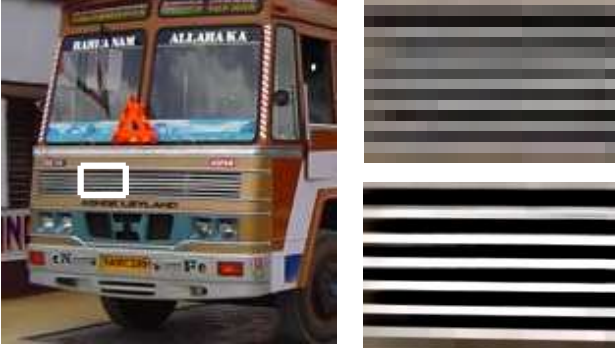
Figure 2. Eight-fold super-resolved reconstruction obtained by our method (bottom right) of an approximately low-rank region (top right and white rectangle on left) in a low-resolution image of a truck (left).
