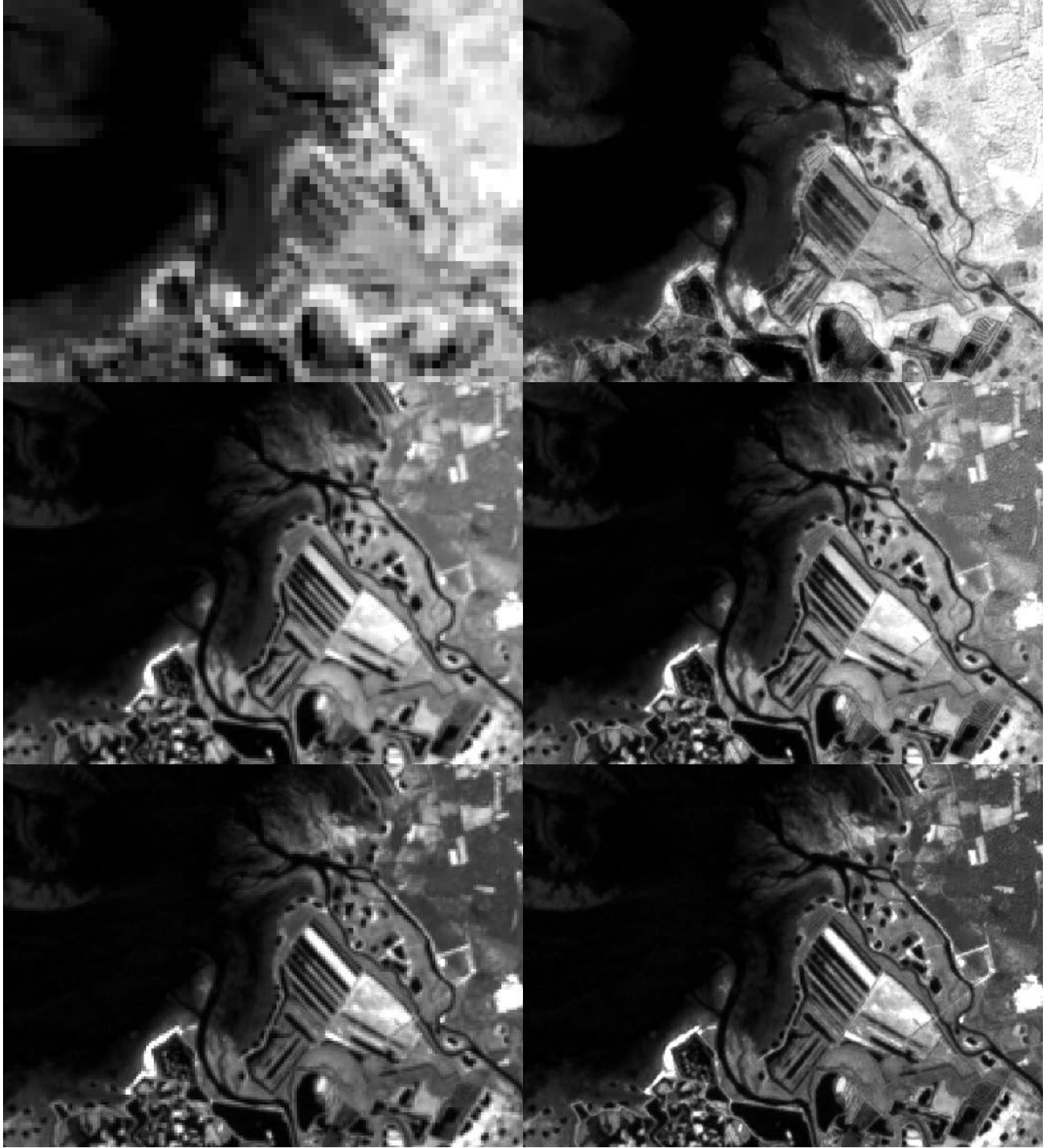
Figure 7. Coastal area (delta of the Leyre river). Top-left: Original band 9 (infrared, 945nm, 60m/pixel). Top-right: Super-resolved band 9 at 10m/pixel. Middle-Left: Original band 11 (deep infrared, 1610nm, 20m/pixel). Middle-Left: Super-resolved band 11 at 10m/pixel. Bottom-left: Original band 12 (deep infrared, 2190nm, 20m/pixel). Bottom-right: Super-resolved band 12 at 10m/pixel.
