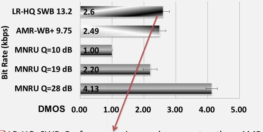
LR-HQ SWB Performance is equal or greater than AMR-WB+ whose algorithmic delay is longer than twice of EVS (32ms)
