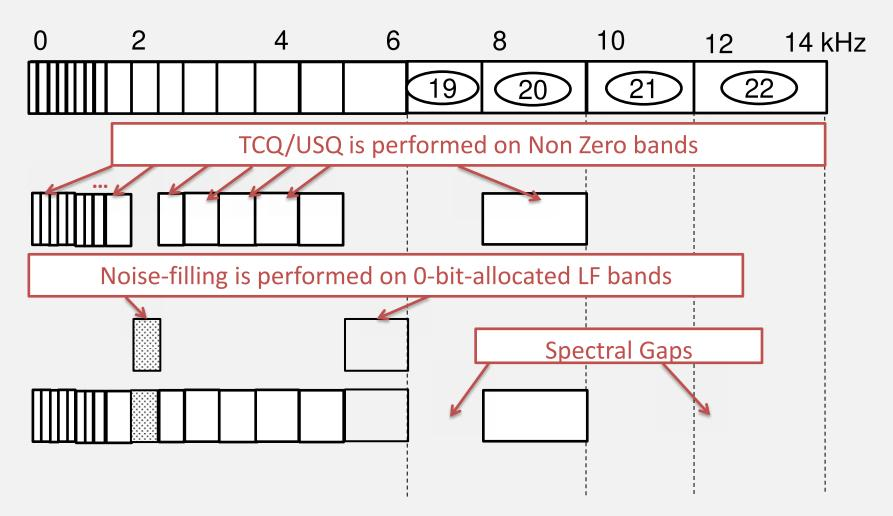
Zero-bit bands cause spectral gaps, which lead to audible artifacts if left alone. Gap filling technique is used.
