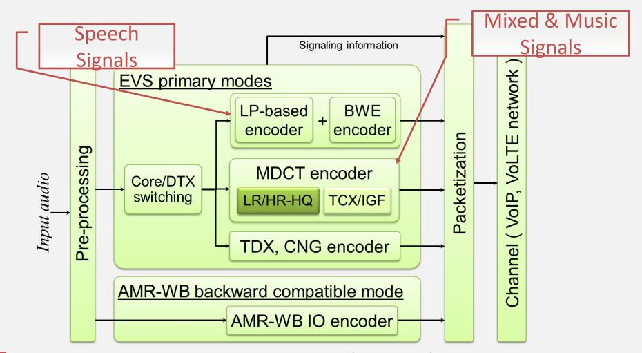
□ The Low Rate High Quality (LR-HQ) MDCT coding is one of the mode in the EVS MDCT coder. 4
