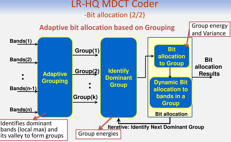
Bits allocated 1) Adaptively grouping the bands and 2) By exploiting the relationship between the groups.
