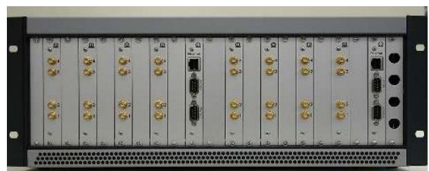
Figure 7: The Supercam real time FFT spectrometer system, built by Omnisys AB. This single 3U crate can process 16 GHz of IF bandwidth at 250 kHz spatial resolution. It consumes less than 200W of AC power.
