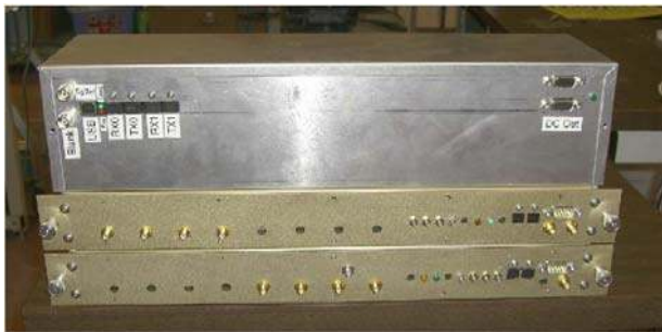
Figure 6: SuperCam IF processor system for two SuperCam rows (16 channels).
