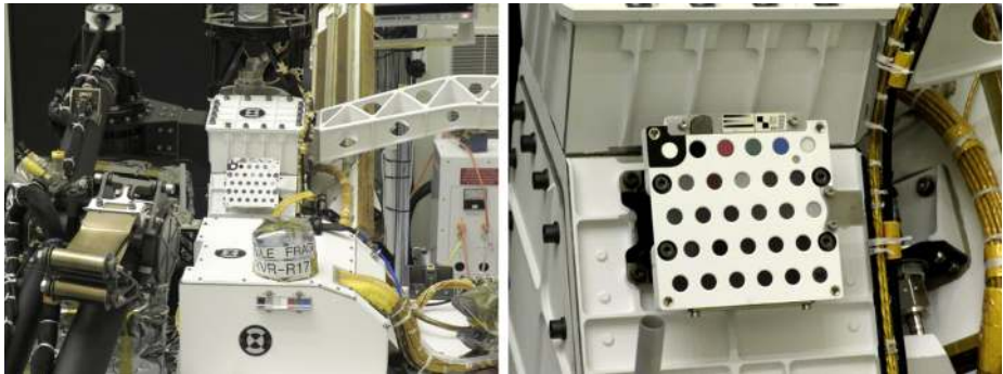
Fig. 1 The SuperCam Calibration Targets are at the rear of Perseverance's deck, on the right side in the forward direction. Photo at Kennedy Space Center. Credits NASA/JPL-Caltech. (Left) An ESD bag is covering the Mastcam-Z primary calibration target; below Mastcam-Z secondary calibration targets
