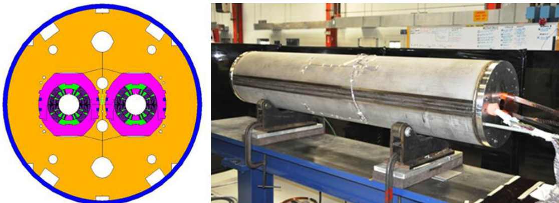
Fig. 30. Cross section of the 11 T two-in-one dipole and picture of the finished 2-m-long cold mass (single bore) ready for testing at Fermilab.
