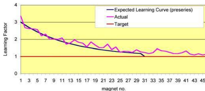
Fig. 7. Learning curve for the total CM production (i.e. collared coils and cold mass finishing, including the welding time) at BNN. Abnormal stop are excluded. Today BNN is welding 4 magnets per week and has shown an extra 25% capacity.
