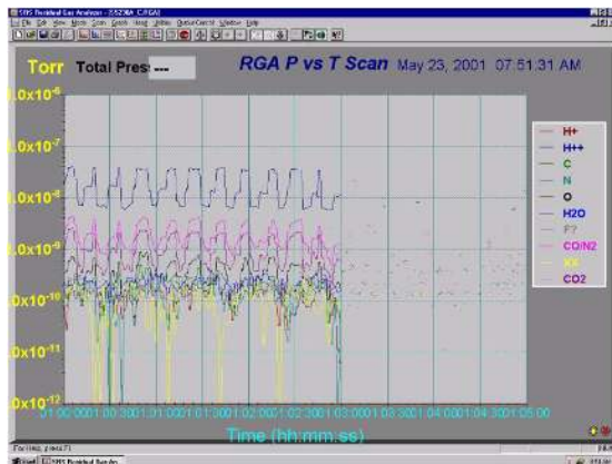
Figure 5: Partial pressure of residual gas species during RF conditioning at 160 – 180 kW.
