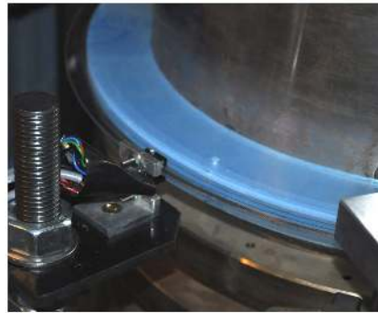
(b) Assembled encoder mounted on armature housing
