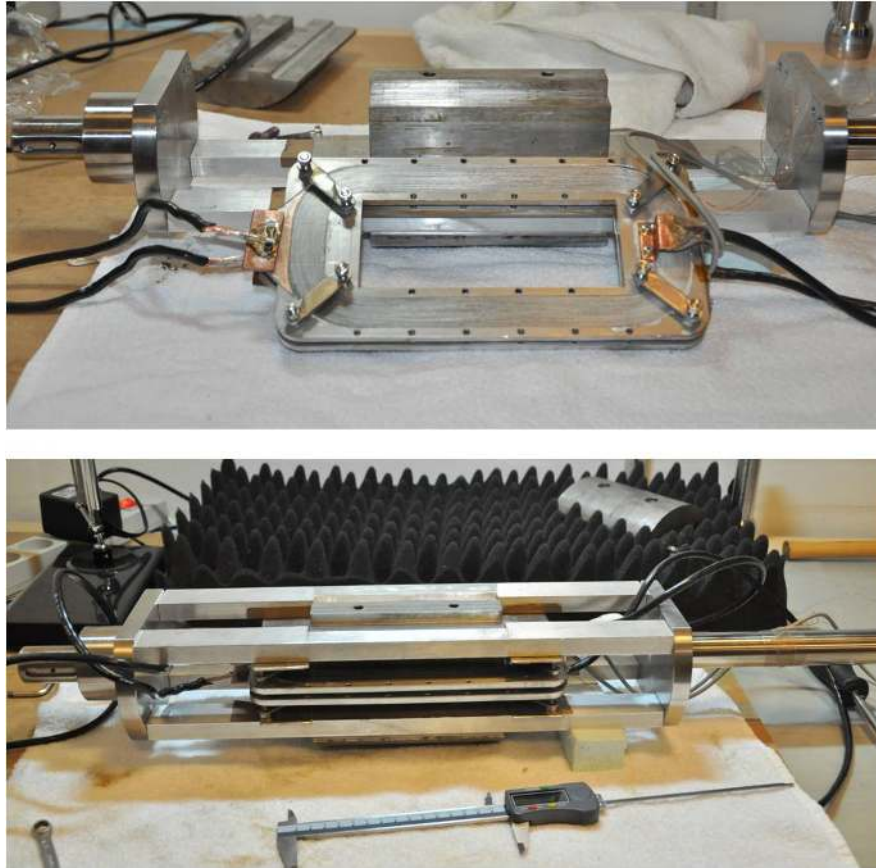
Figure 4.15: HTS field winding - The HTS field winding is shown in assembly phase with two HTS coils mounted on the cold steel.
