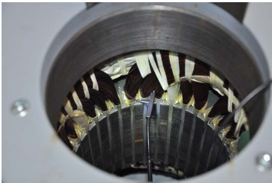
Figure 4.4: Placement of the Rogowski current transducer. - The transducer is wrapped around turns placed in two armature slots.
