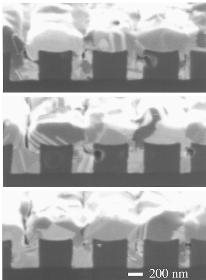
Figure 11. FIB image of copper deposited from the additive-free electrolyte ( -0.563 V for 45 s). Three different groups from the same sample are shown. From left to right the trench width ranges from 370 to 110 nm while the aspect ratio varies from 1.1:1 to 3.8:1. Note that the shape of the void changes from a circle to an elongated seam as the trench becomes narrower. The seam corresponds to \sim 10\% of the trench width as anticipated by published simulations. 34
