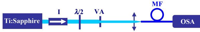
Figure 36. Experimental setup for dispersion measurement using the spectral modulation effect. I: isolator, \lambda/2 : half-wave plate, VA: variable aperture, and OSA: optical spectrum analyzer.
