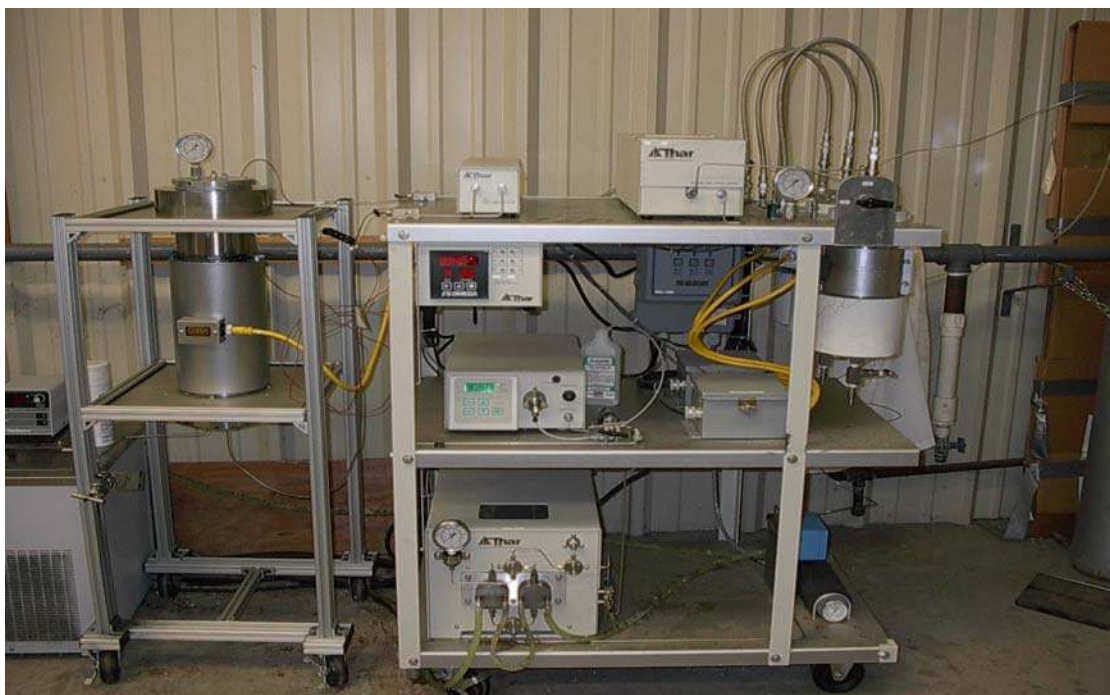
Figure 3.3.1 Pilot scale supercritical fluid extractor used for the experiments
