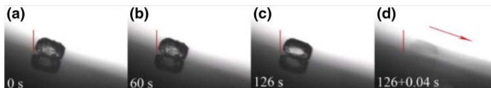
Fig. 11: Deliquescence of an NaCl particle on tilted superhydrophobic surface in an atmospheric condition of RH = 90% after (a) 0 s, (b) 60 s, (c) 126 s, and (d) 126 + 0.04 s 68
