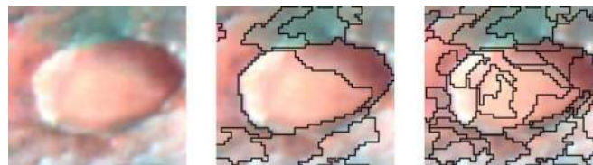
Fig. 1. Segmentation of an image patch from CRISM frt00003e12, originally from [4] ( R : 2.0 \mu\text{m}, G : 1.5 \mu\text{m}, B : 1.1 \mu\text{m} ). (Left) Original subimage. (Center) Coarse segmentation, minimum region size 100. (Right) Fine segmentation, minimum region size 20. Finer segmentations provide additional resolution at the cost of greater computation time and sensitivity to noise. Image courtesy NASA / John Hopkins.
