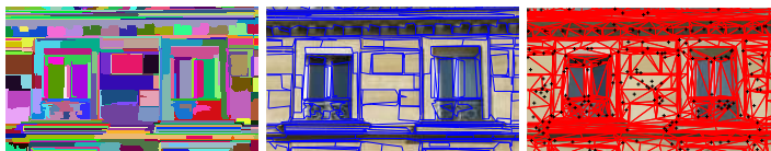
Figure 3: One way of obtaining a 2D base mesh: superpixelization (left), boundary polygonization (middle), constrained Delaunay-triangulation (right).
