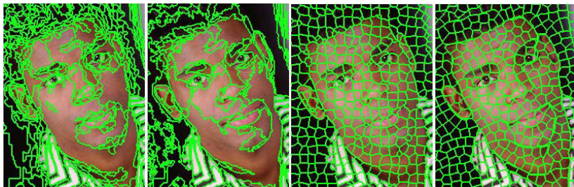
Fig. 1. From left to right: meanshift [11], graph based [12], turbopixels [14], NC superpixels [1]. Implementation was obtained from the authors’ web sites.
