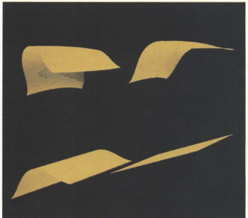
Figure 12. Progressive deformation of a rectangular flat sheet. Vector bundles are differentially rotated to produce the new forms.
