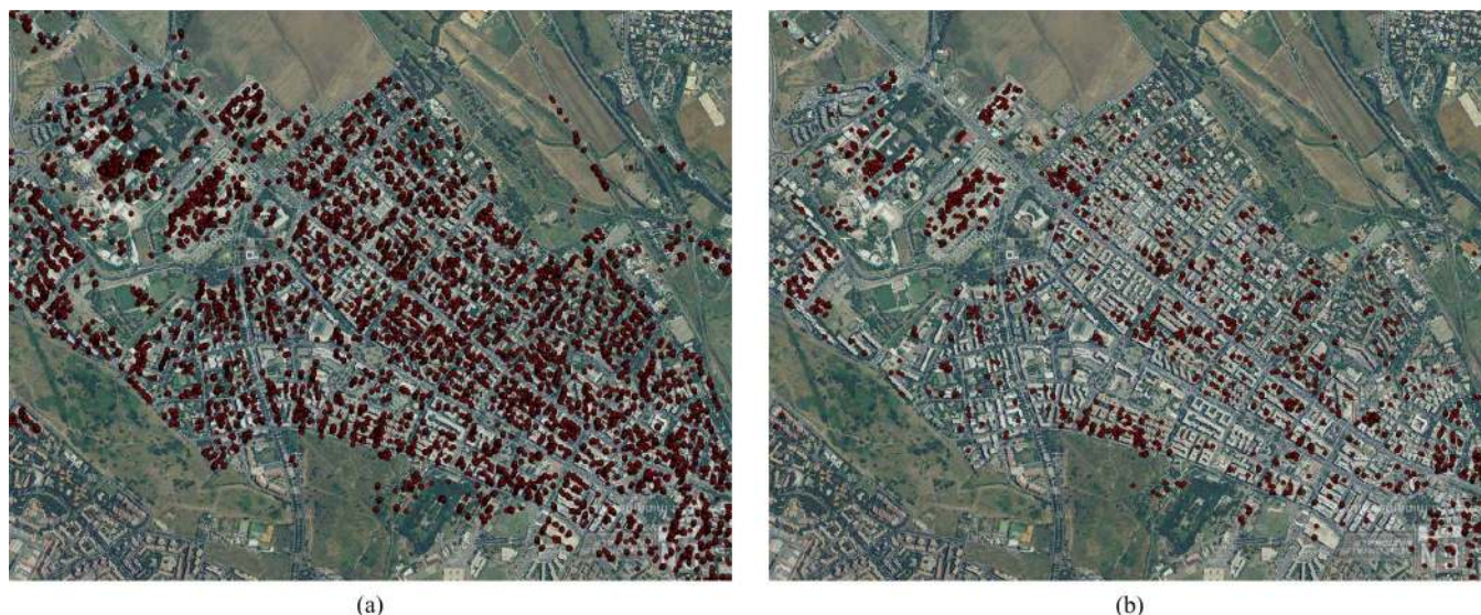
Fig. 16. (Dark red dots) Geocoded positions of the scatterers detected with the Rome data set. (a) Single scatterers. (b) Dominant double scatterers.
