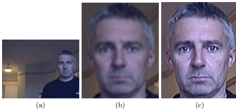
Figure 17: Superresolution of a full video sequence (frame size 160x120 pixels) (a) Interpolated LR frame; (b) BSR result
