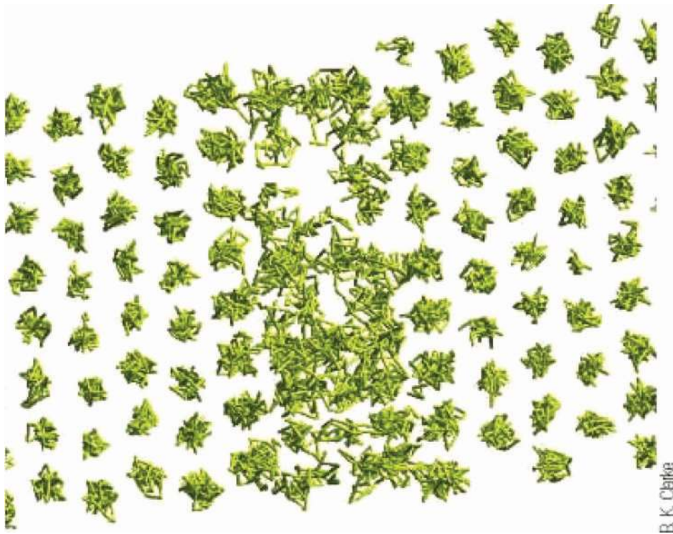
Figure 6. As shown by this numerical simulation by B. Clark and D. Ceperley [39], a grain boundary is a fluid layer a few atomic layers thick.
