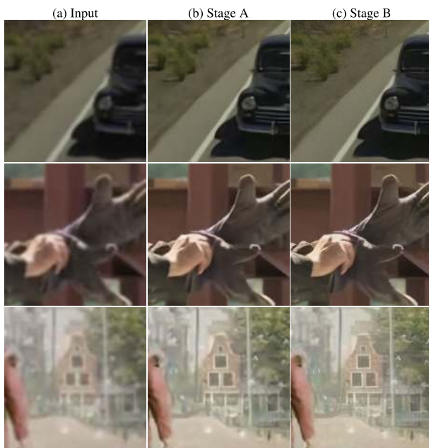
FIGURE 12. Relevance of components in SUPERVEGAN-4. After the stage A (Fig. 12b) block artifacts are removed and image is 2x upscaled. After the stage B (Fig. 12c) the image is upscaled to 4x; sharpness and fine details are added.
