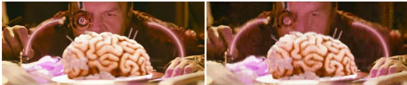
FIGURE 1. From a low bitrate (250Kbps) and low resolution (320 × 180px) input video, our method reduces artifacts and achieves high resolution (1280 × 720px) (left), compared with the original video compressed at the same bitrate with H264 (right). Image is taken from [2].
