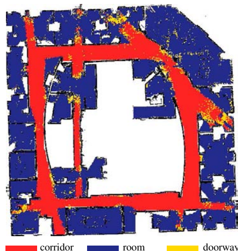
Fig. 8. Classification results obtained by applying the classifier learned for the environment depicted in Figure 1 to the map of the Intel Research Lab in Seattle. The fact that 82.23% of all places could be correctly classified illustrates that resulting classifiers can be applied to so far unknown environments.
