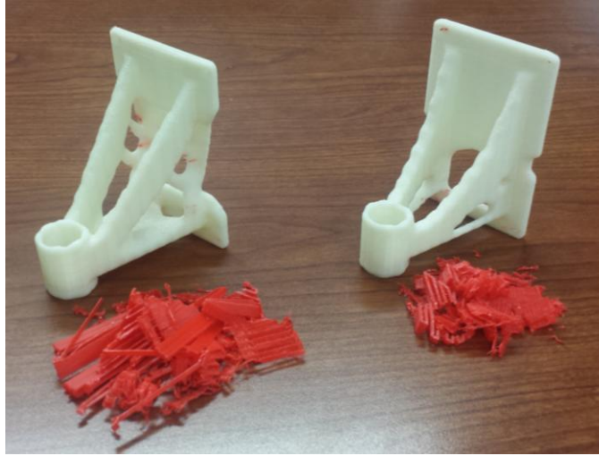
Figure 25: Printed mount bracket and the required support structures at 0.7 volume fraction.
