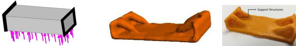
Figure 2: (a) Structural problem. (b) Optimized topology. (c) Fabricated part with support structures.
