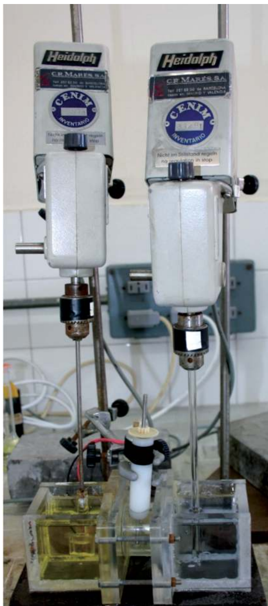
Figure 1. View of a sandwich-membrane type cell. Left hand compartment is for the feed solution, middle compartment is for the organic solution, right hand compartment is for the stripping solution. Two solid supports are located between the feed and organic and the organic and stripping phases compartments, respectively. The three compartments are stirred in order to homogenize the respective bulk solutions.
