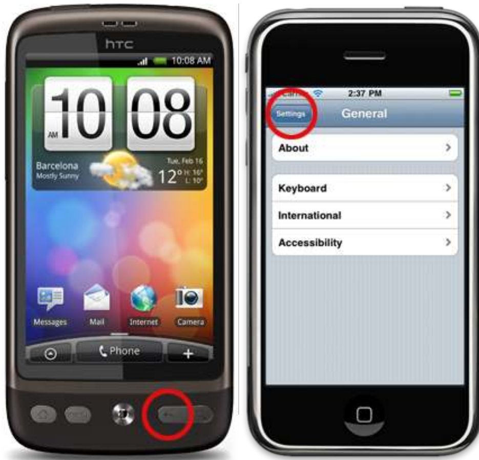
Figure 3.1: Different platforms have different standard solutions for commonly used features like back buttons. Web applications must embrace these solutions and not create their own standards
