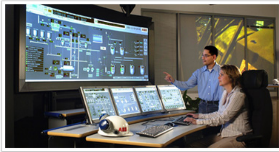
Figure 1.1: Operators working in the process automation industry uses control systems that usually runs on several screens
