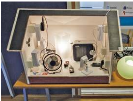
Figure 13: A small scale model of a Smart House based on the architecture shown in Figure 12.
