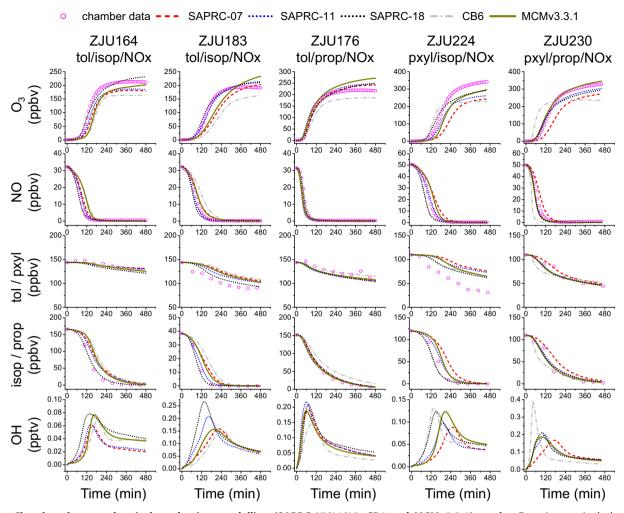
Fig. 2 Chamber data vs. chemical mechanism modelling (SAPRC-07/11/18, CB6 and MCMv3.3.1) results. Experiments include toluene/isoprene/ $NO_x$  (ZJU164/183), toluene/propene/ $NO_x$  (ZJU176), p-xylene/isoprene/ $NO_x$  (ZJU224) and p-xylene/propene/ $NO_x$  (ZJU230).
