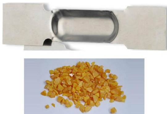
Figure 3.1: Notched boat employed in STF-deposition experiments and ZnSe in granular form [61, 62]
